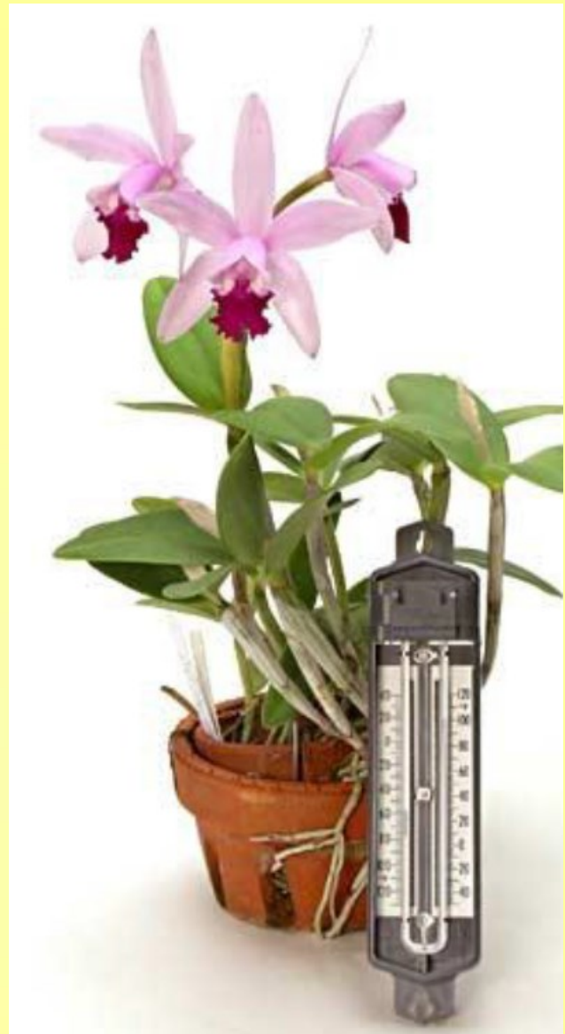
A min-max thermometer will show you the temperature range over a given period of time.
