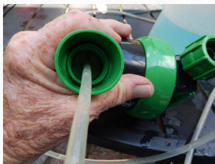
Take a length of Fish tank airline hose and just stick it down into a bottle of your solution and stick the other end on the little nozzle inside the fertilizing bottles receiver attachment.
